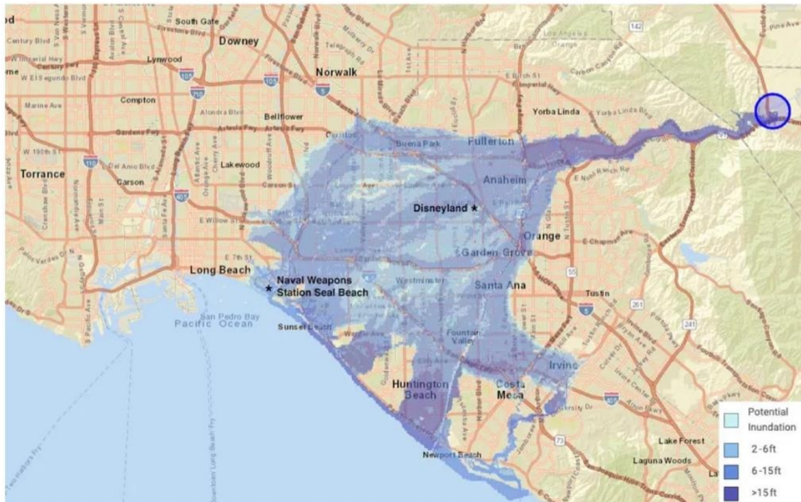
Figure 5. Potential worst-case inundation from a breach of the Prado Dam in California. Water depths in excess of six feet would be possible over a large swath of the eastern Los Angeles area, with a few isolated areas with inundations exceeding 15 feet. (Image credit: USACE ).
